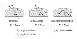
In the **MA886** refractometer, light from an LED passes through a prism in contact with the sample. An image sensor determines the critical angle at which the light is no longer refracted through the sample.
