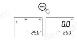
Gently absorb the ZERO water standard with a soft tissue. Use care not to scratch the prism surface. Dry the surface completely. The instrument is ready for sample measurement.
